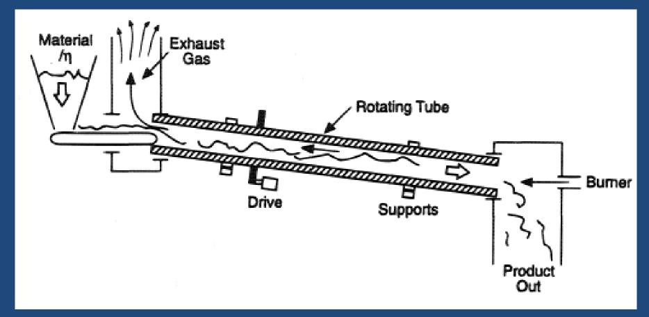
Cross section of a typical rotary kiln
